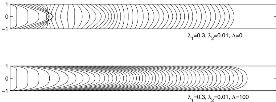
Fig. 5. Velocity profiles shifted in time in SU flow. Comparison between cases (b) and (c).
