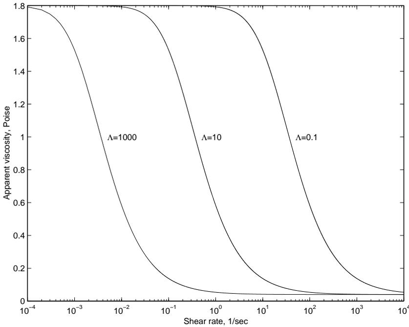
Fig. 1. The shear rate dependent viscosity function (3.3) with  $\eta_0 = 180$  cP,  $\eta_\infty = 4$  cP for three values of  $\Lambda$  (in sec).
